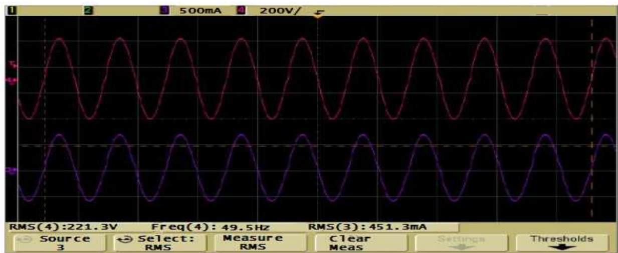
Figure 13. Output Voltage and Current (100W Load)
