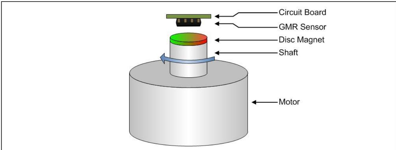
**Figure 1** Example GMR sensor application
