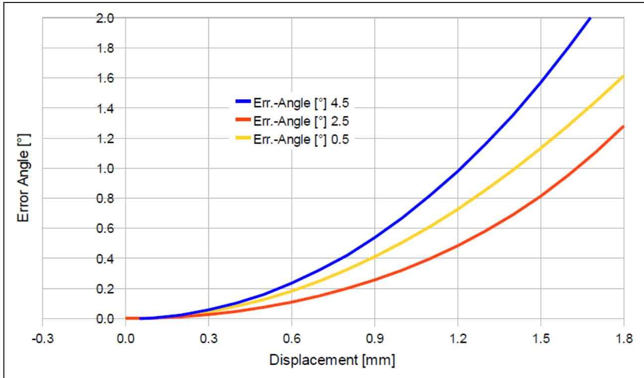
**Figure 13** Maximum error angles associated with different air gaps
