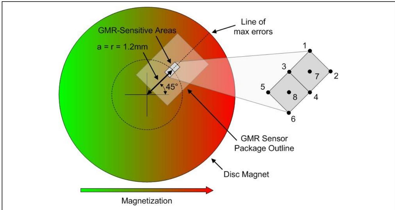
**Figure 17 Configuration for evaluation of the field distribution across the two sensor areas**
