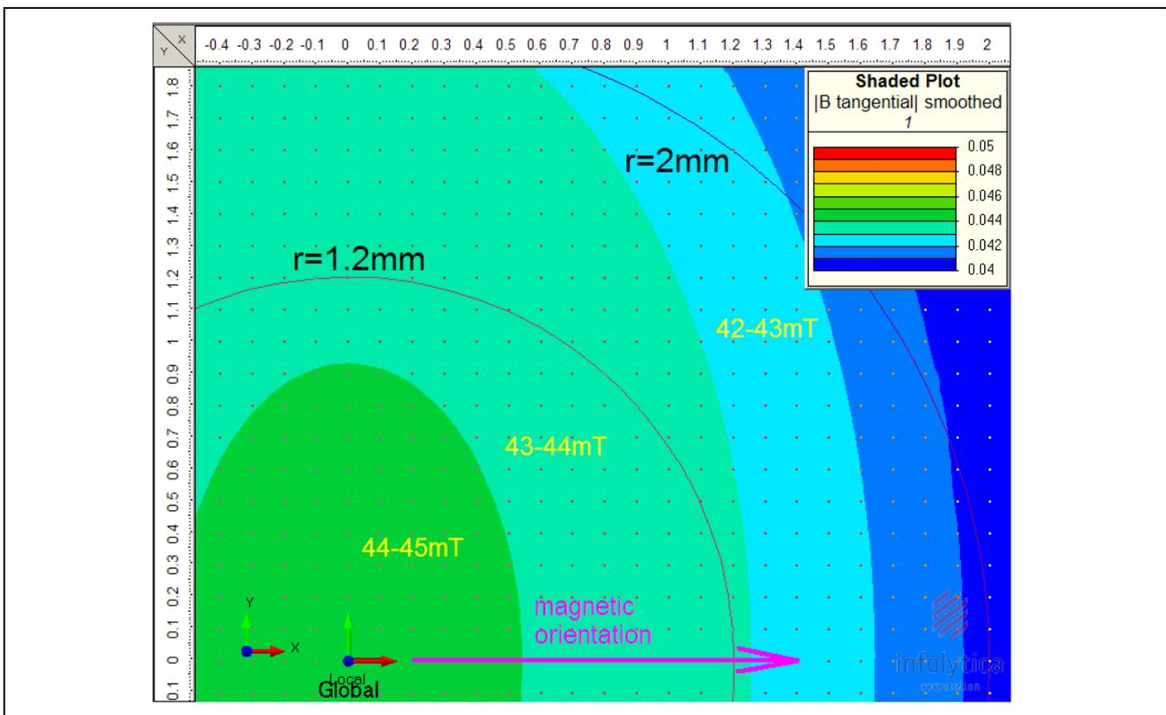
Figure 15 Distribution of tangential induction in the *Bx-By* plane with an air gap of 2.5mm
