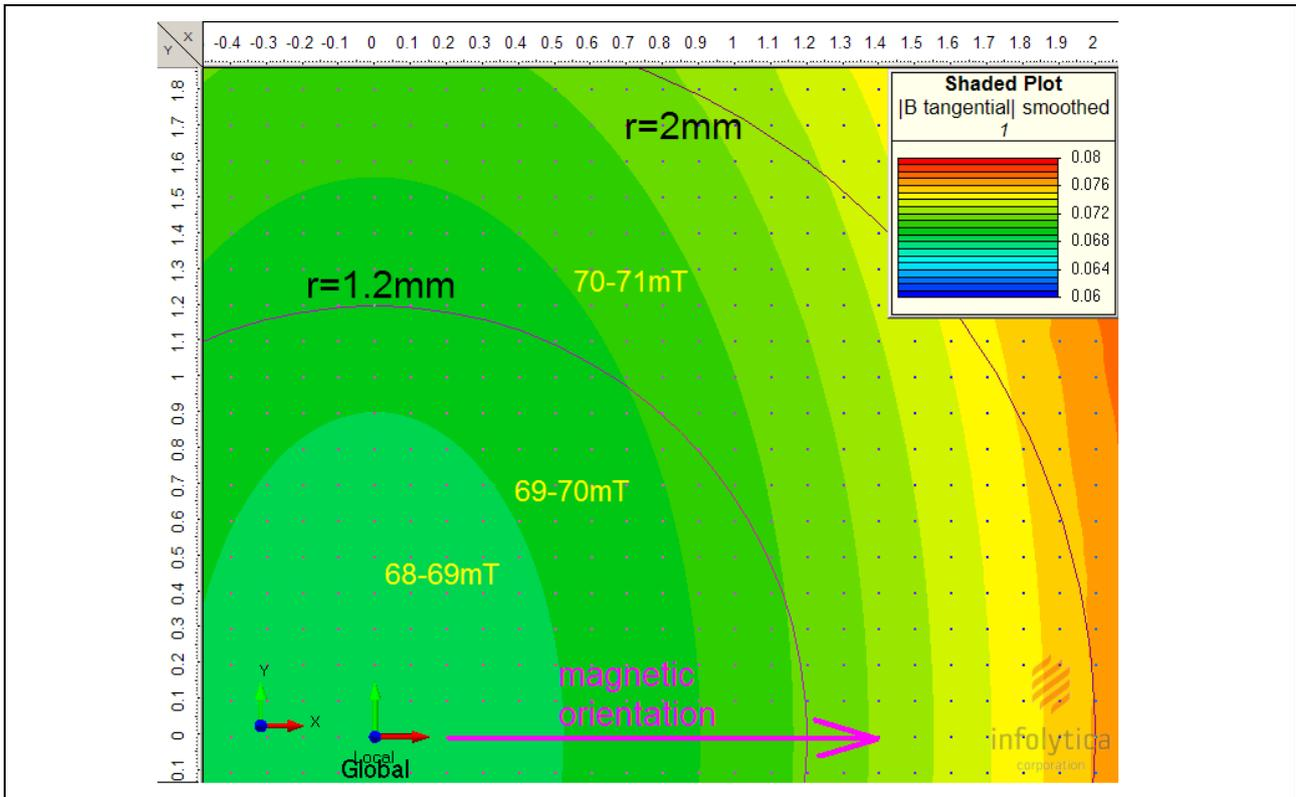
Figure 14 Distribution of tangential induction in the *Bx-By* plane with an air gap of 0.5mm
