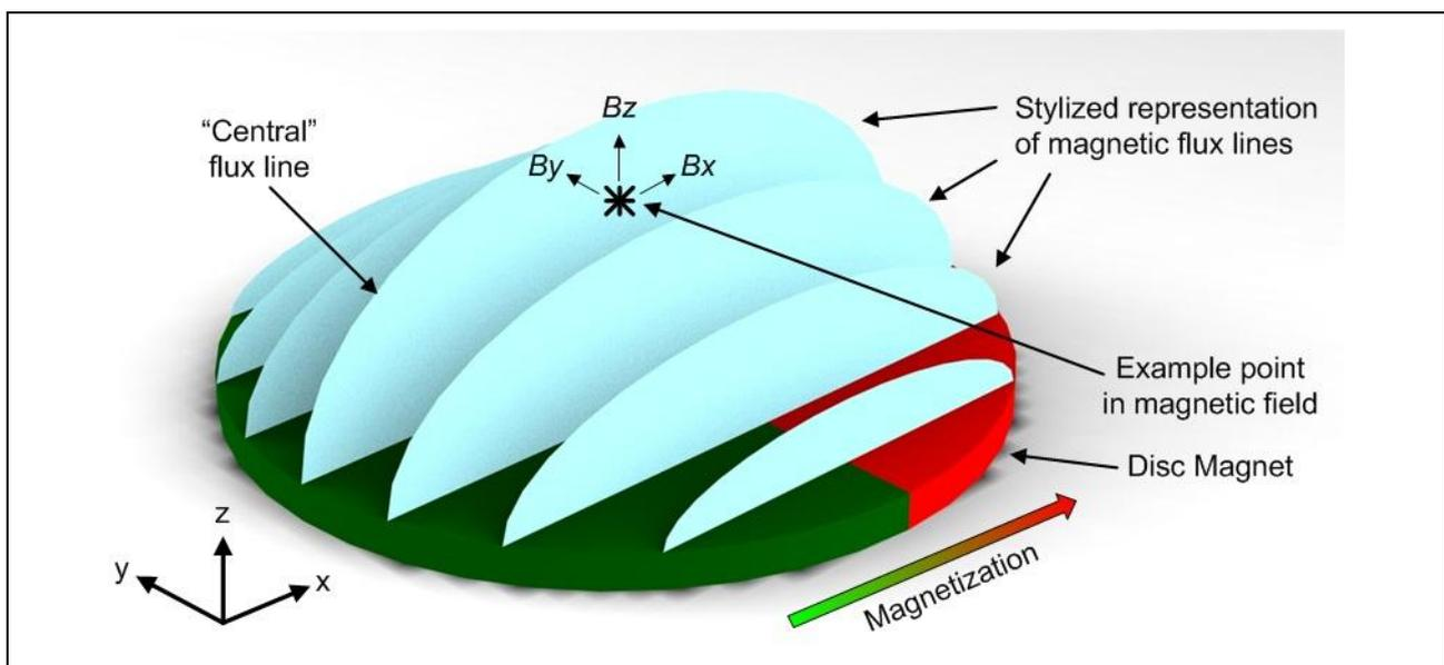
**Figure 6** Stylized representation of an ideal magnetic field
