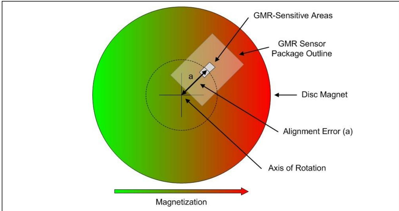
**Figure 5** Top view of GMR-sensitive areas displaced (misaligned) with respect to the axis of rotation
