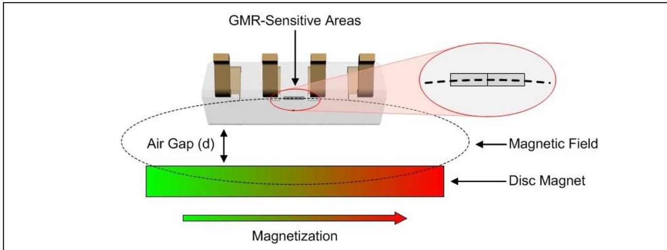
**Figure 3** Side view of the sensor package relative to the disc magnet
