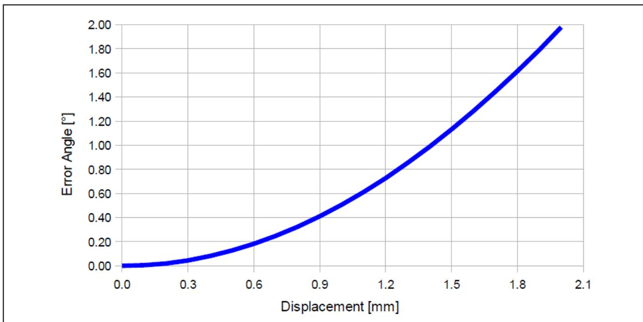
**Figure 12** Maximum error angles associated with increasing displacement from the axis of rotation
