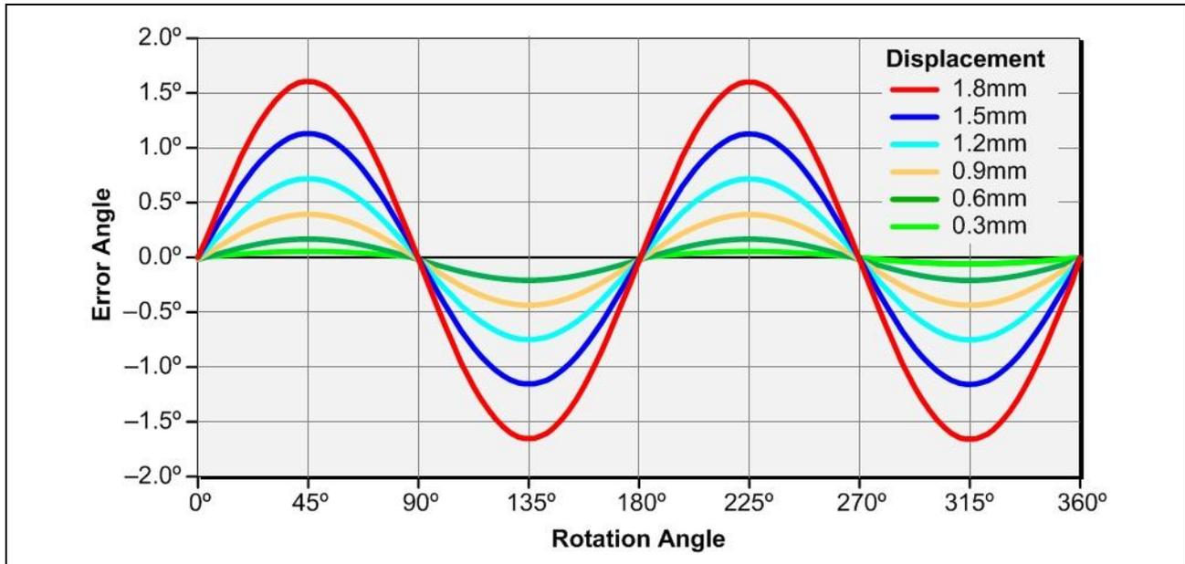
**Figure 11** Resulting error angles associated with increasing displacement from the axis of rotation
