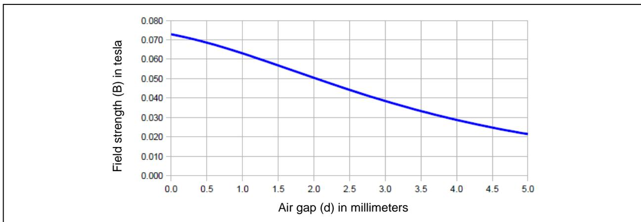
**Figure 9** Variation of flux density  $B$  on the rotation axis of the proposed disc magnet at  $20^{\circ}\text{C}$
