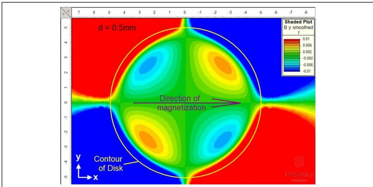
**Figure 10** Distribution of  $B_y$  components in a plane 0.5mm above the surface of the disc magnet
