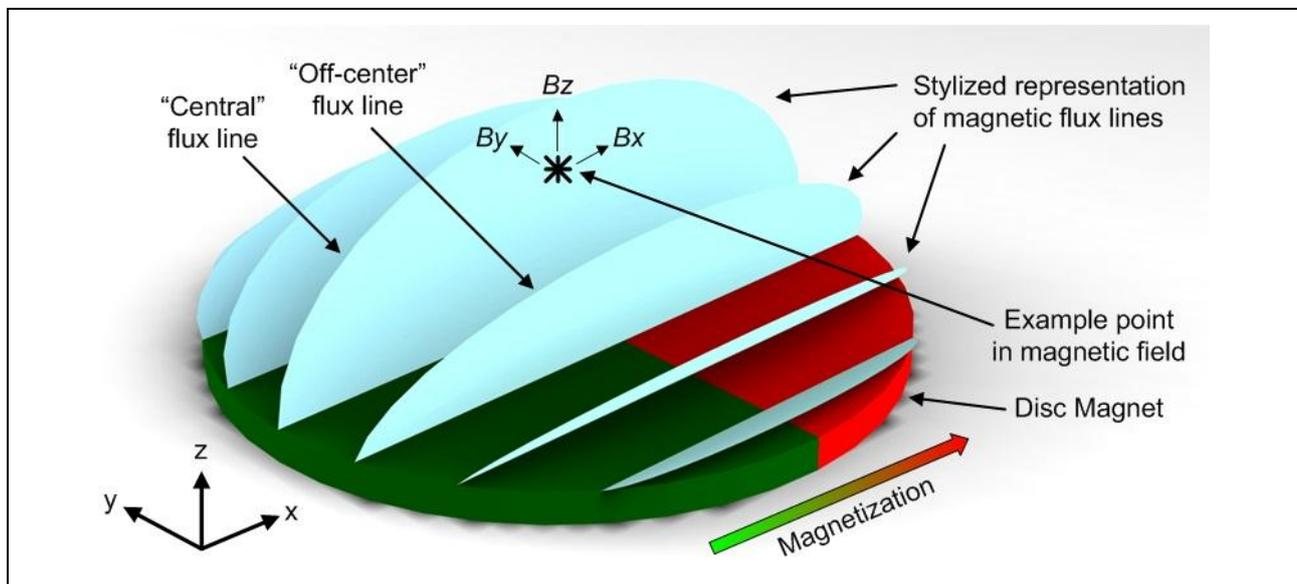
**Figure 7 Stylized representation of realistic magnetic field**
