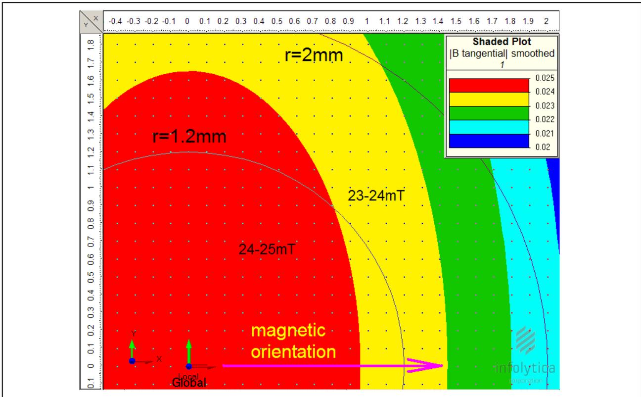
**Figure 16** Distribution of tangential induction in the  $B_x$ - $B_y$  plane with an air gap of 4.5mm
