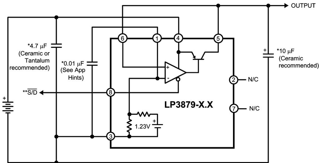
\*Capacitance values shown are minimum required to assure stability. Larger output capacitor provides improved dynamic response. Output capacitor must meet ESR requirements (see Application Information).
