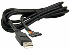
FTDI 3.3V cable, available from Adafruit.com
