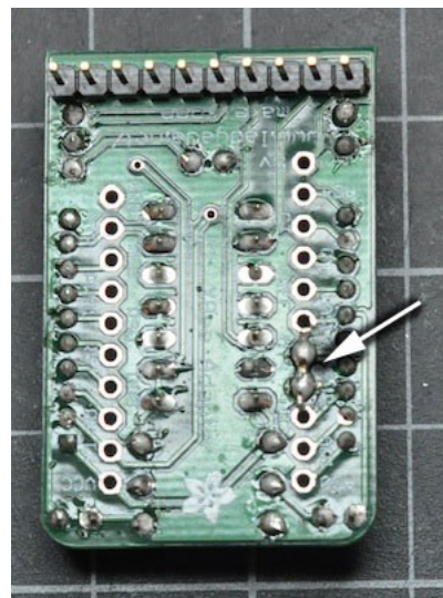
Modified Adafruit XBee Adapter Kit The arrow shows the added solder connection
