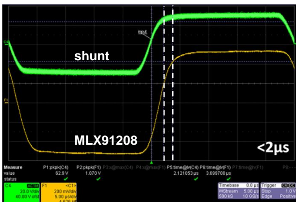
Figure 12: Response time with noise filter OFF.
